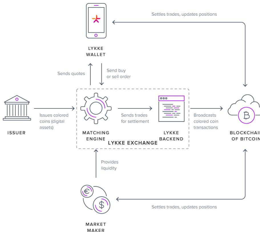
Figure 7: Lykke Exchange high-level architecture
